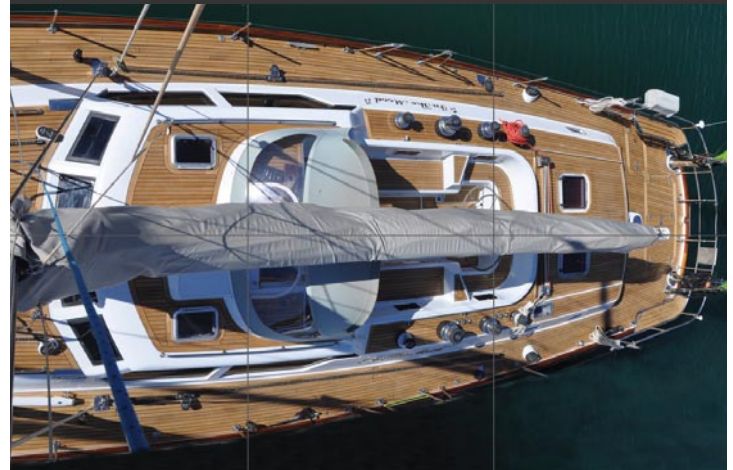
Oyster 72 "In the Mood" teak decks, re-laid and refurbished
